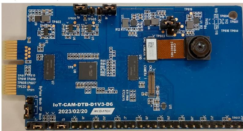
Figure 4-4. D6 Camera Board
